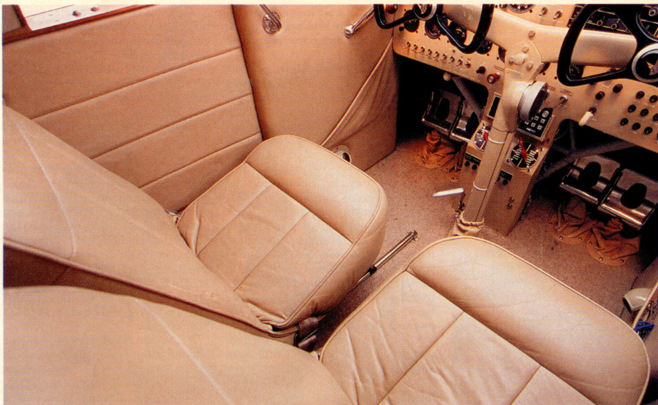
Inside this prize-winning Staggerwing is a leather interior with room for five. A modified fuel system places the selectors on the center pedestal.
