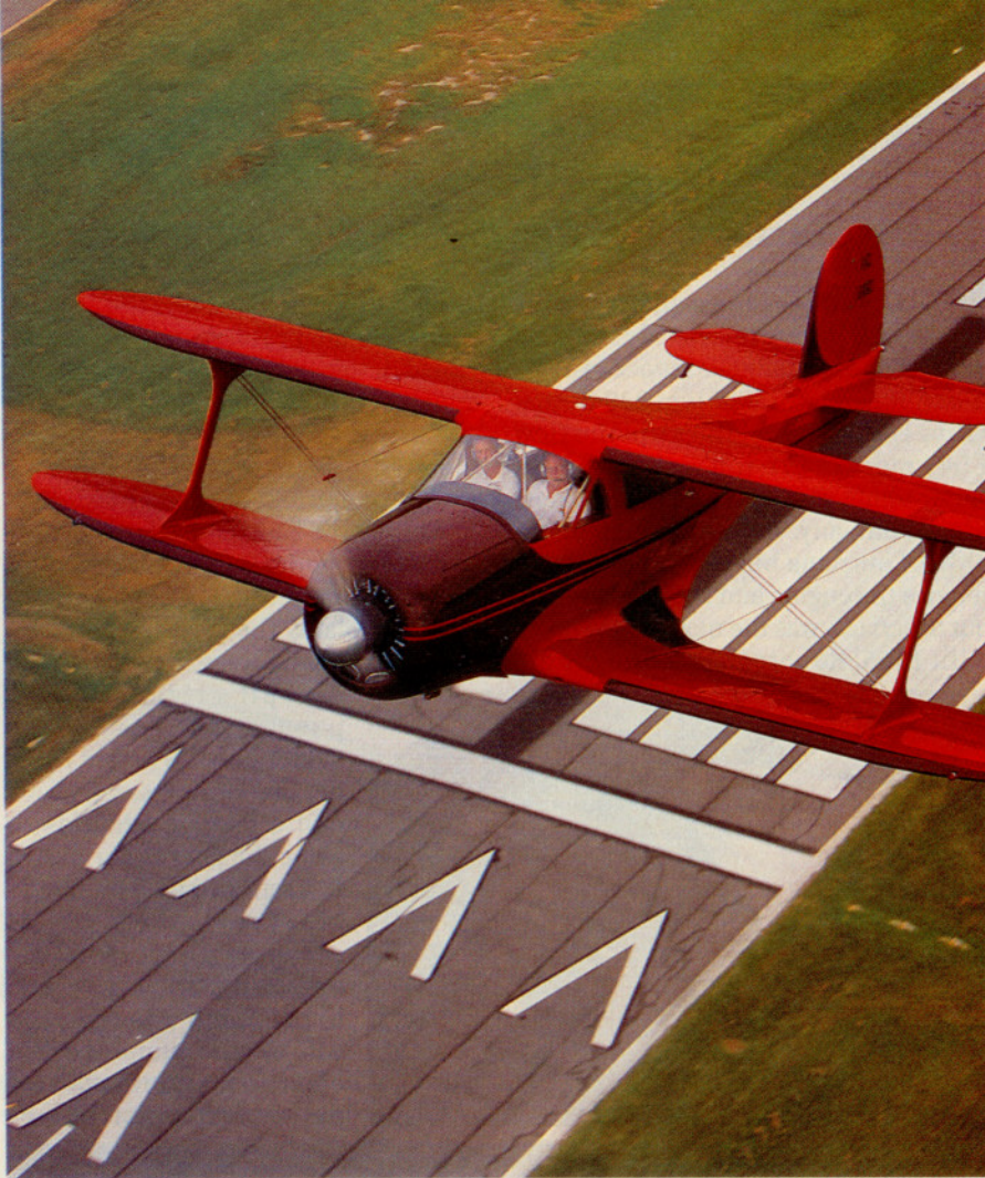
Runway performance is not a problem with 450 hp pulling the 4,200-pound Staggerwing (above). Oreck's G17S was converted from a basket-case D17S to an Oshkosh Grand Champion.
