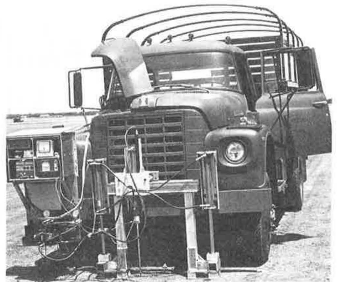
FIGURE 3 Automated penetrometer ready for testing operation.
