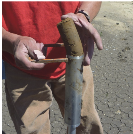
Figure 31. Trimming the soil sample.
