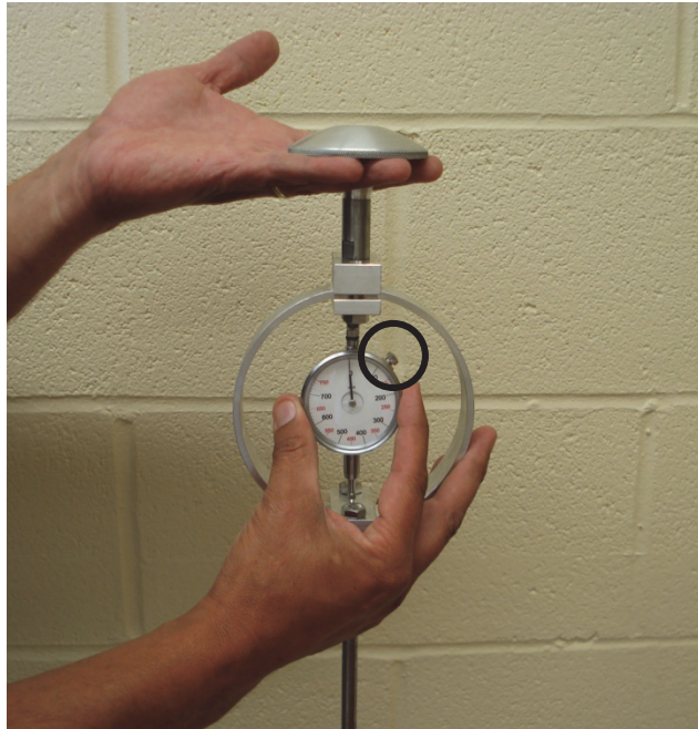
Figure 20. Zeroing the gage.
