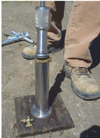
Figure 34. Pressing remold sample into place.
