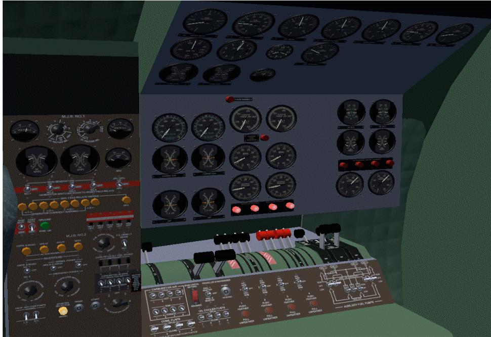
*Figure 25 - engine instruments in normal range*
