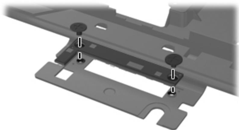
**Where used:** 2 screws that secure the button board to the switch cover
