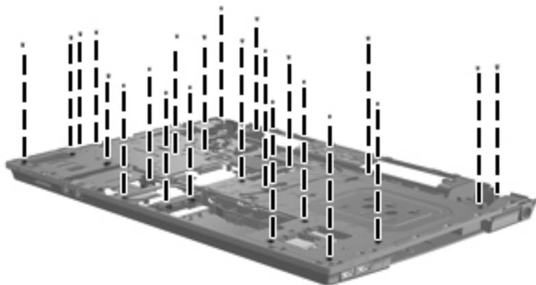
**Where used:** 22 screws that secure the top cover to the base enclosure.
