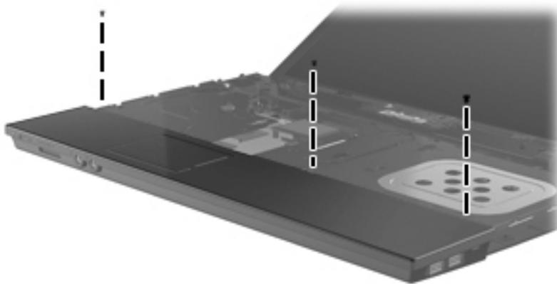
**Where used:** 3 screws that secure the palm rest to the computer
