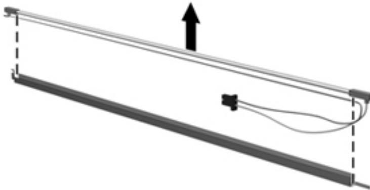
18. Disconnect the display panel cable (1) from the LCD panel.
