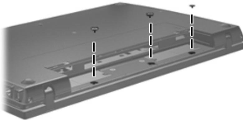
**Where used:** 3 screws that secure the switch cover to the base enclosure
