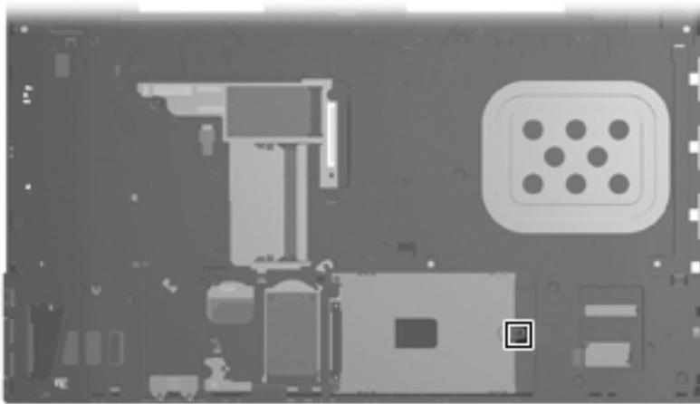
**Where used:** One captive screw that secures the hard drive to the computer (screw is secured to the hard drive bracket)
