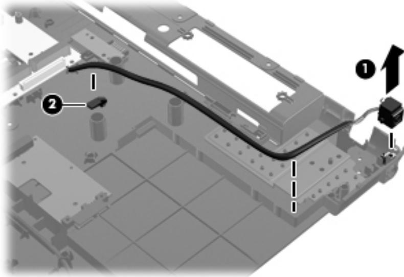
3. Remove the battery connector board (1).
