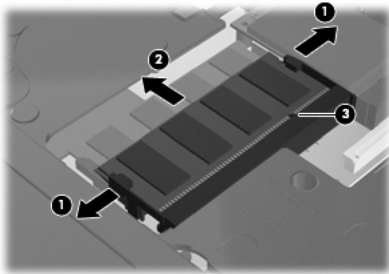
Reverse this procedure to install a memory module.
