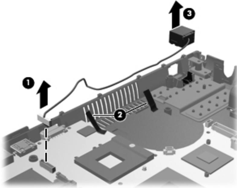
Reverse this procedure to install the RJ-45 (network) jack.
