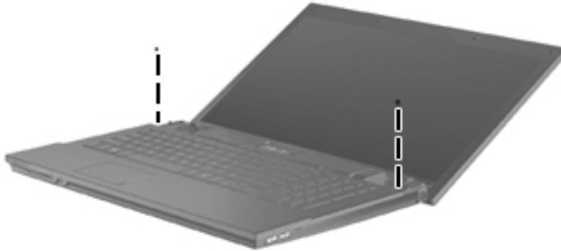
6. Slide the keyboard back (1), and rotate it forward (2) until it rests on the base enclosure.
