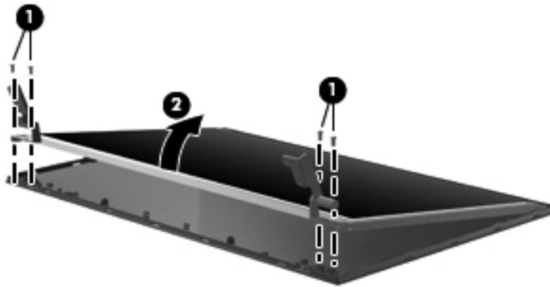
10. Remove the four Phillips PM2.0×3.0 screws (1) that secure each display hinge to the display panel.
