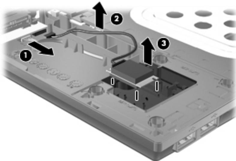
Reverse this procedure to install the Bluetooth module.
