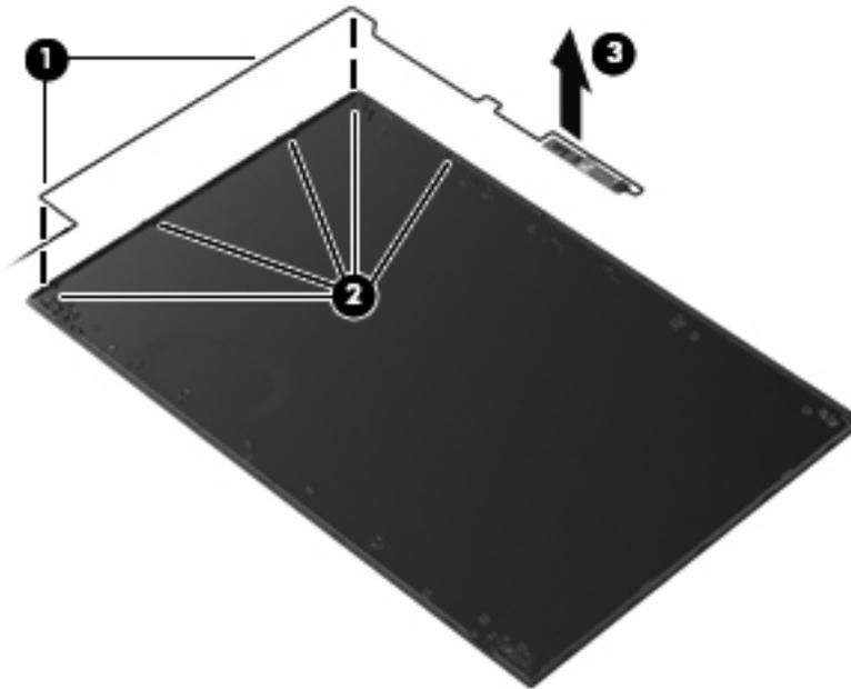
16. If it is necessary to replace the microphone, lift the microphone from the clip (1) and gently pull the microphone cable from the routing channels (2). The microphone cable is included in the Display Cable Kit, spare part number 535771-001
