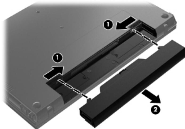
Install the battery by inserting it into the battery bay until you hear a click.
