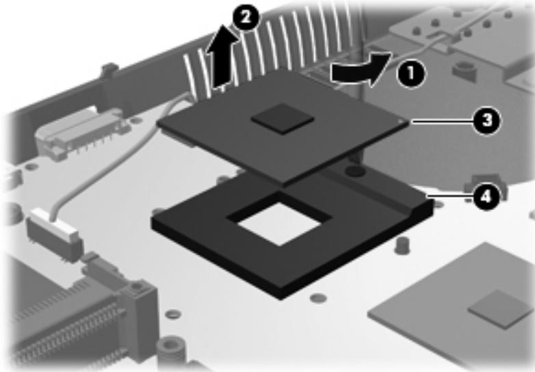
Reverse this procedure to install the processor.
