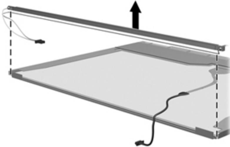
17. Remove the backlight from the backlight frame.
