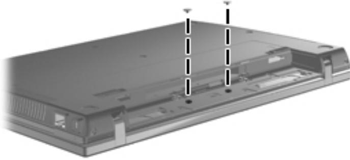
**Where used:** 2 screws that secure the top cover and battery connector board to the base enclosure
