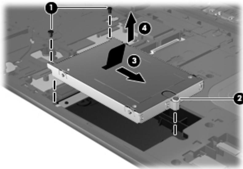
6. If it is necessary to replace the hard drive bracket, remove the two Phillips PM3.0×4.0 hard drive bracket screws (1) from each side of the hard drive.
