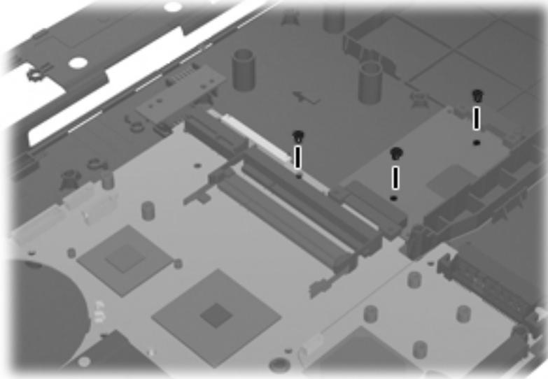
**Where used:** 3 screws that secure the system board to the base enclosure
