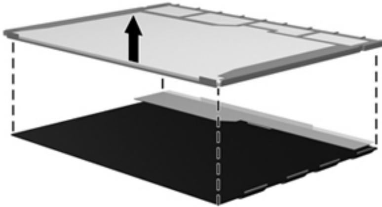
23. Recycle the LCD panel and backlight.
