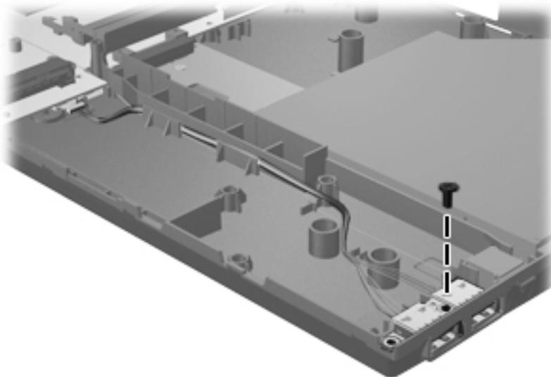
**Where used:** One screw that secures the USB board to the system board
