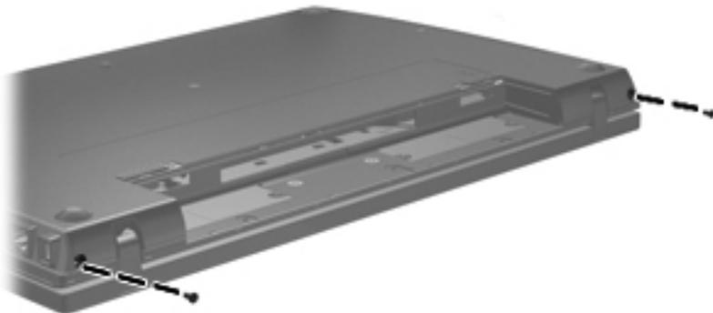
**Where used:** 2 screws that secure the switch cover to the computer
