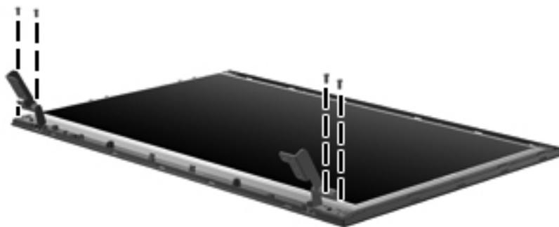
**Where used:** 4 screws that secure the display panel to the display assembly
