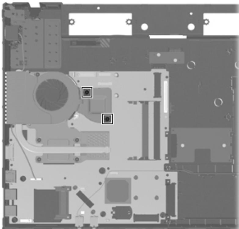
**Where used:** 2 captive screws that secure the heat sink to the computer
