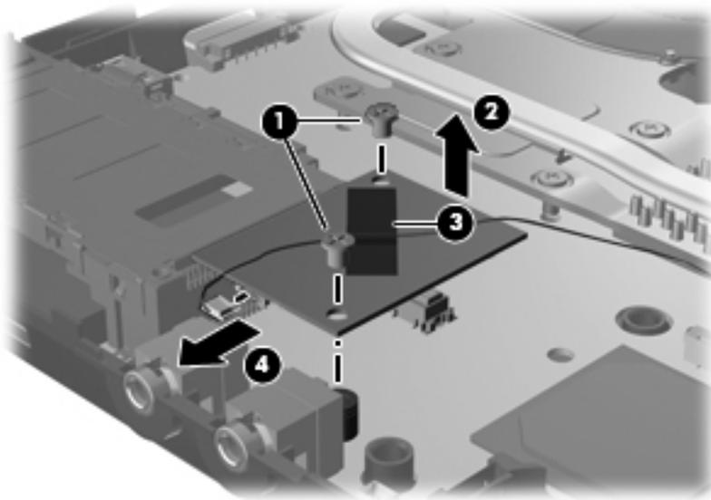
4. Remove the modem module.
