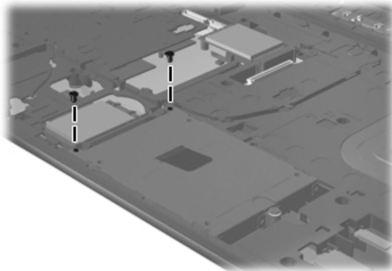
**Where used:** 2 silver screws that secure the hard drive to the top cover
