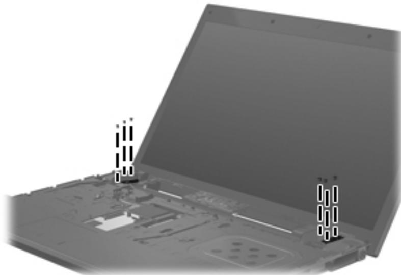
**Where used:** 6 screws that secure the display assembly to the computer.
