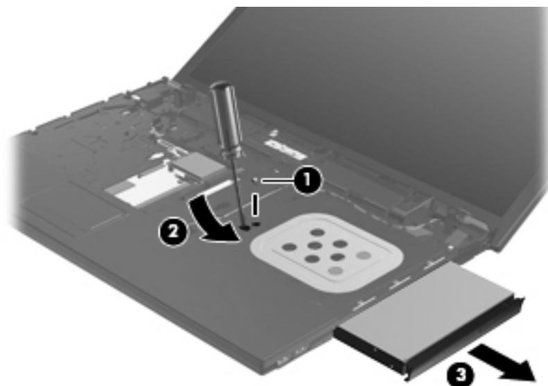
5. If it is necessary to replace the optical drive bracket, position the optical drive with the rear toward you.
