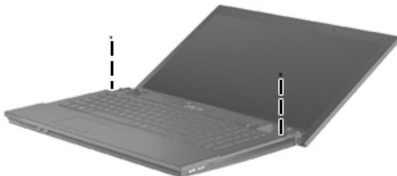
**Where used:** 2 screws that secure the keyboard to the computer
