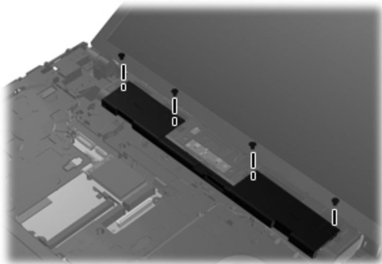
**Where used:** 4 screws that secure the speaker assembly to the computer
