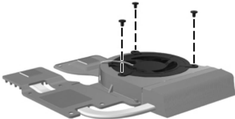
**Where used:** 3 screws that secure the fan to the heat sink
