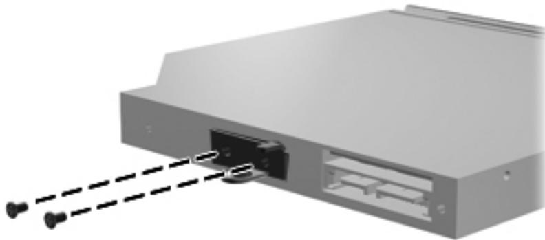
**Where used:** 2 screws that secure the optical drive bracket to the optical drive
