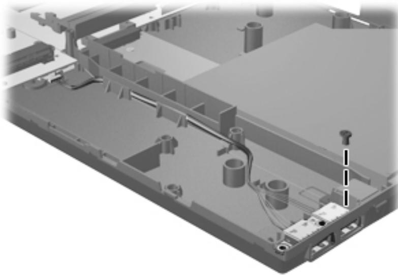
Where used: 1 screw that secures the USB board to the computer
