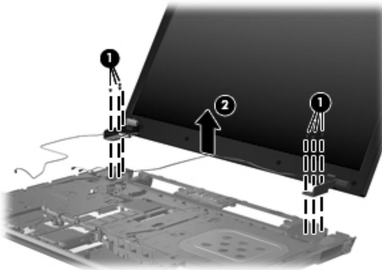
2. If it is necessary to replace the display bezel or display hinges, remove the eight rubber screw covers (1) and the eight Phillips PM2.5×4.5 screws (2) that secure the display bezel to the display assembly. The rubber screw covers are available in the Rubber Kit, spare part number 535793-001.
