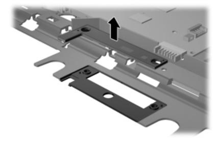
Reverse this procedure to install the power button board.
