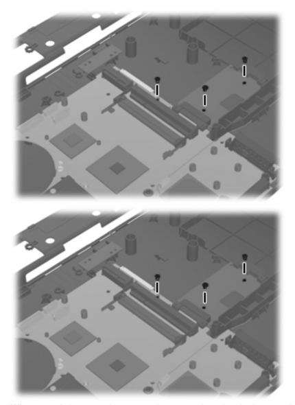
Where used: 3 screws that secure the system board to the base enclosure
