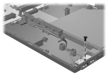
Where used: One screw that secures the USB board to the system board
