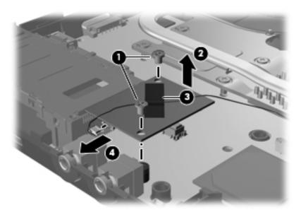
4. Remove the modem module.
