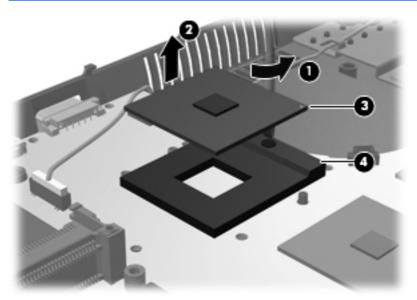
Reverse this procedure to install the processor.
