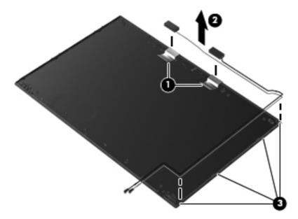
15. If it is necessary to replace the webcam, gently pull the webcam cables (1) from the clips and routing channels (2) built into the top cover. Lift the webcam (3) to remove it. The webcam cable is included in the Display Cable Kit, spare part number 535771-001.
