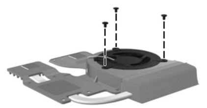
Where used: 3 screws that secure the fan to the heat sink
