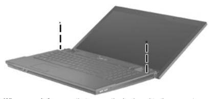
Where used: 2 screws that secure the keyboard to the computer
