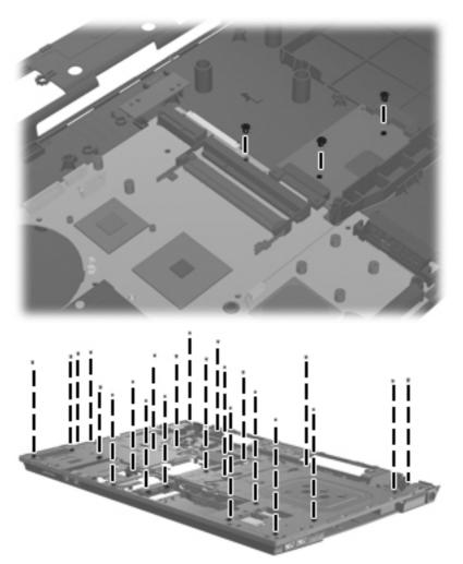
Where used: 22 screws that secure the top cover to the base enclosure.
