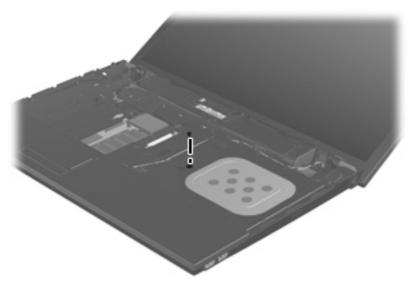
Where used: 1 screw that secures the optical drive to the computer
