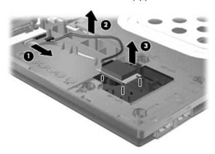
Reverse this procedure to install the Bluetooth module.
