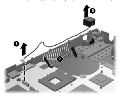
Reverse this procedure to install the RJ-45 (network) jack.
