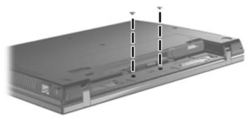
Where used: 2 screws that secure the top cover and battery connector board to the base enclosure
