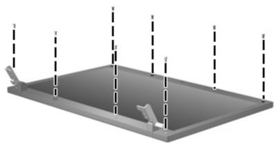
Where used: 8 screws that secure the display bezel to the display enclosure
