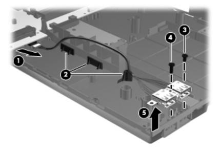
Reverse this procedure to install the USB connector module.
