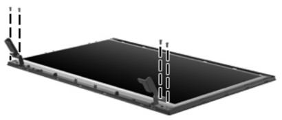
Where used: 4 screws that secure the display panel to the display assembly
