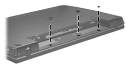
Where used: 3 screws that secure the switch cover to the base enclosure
