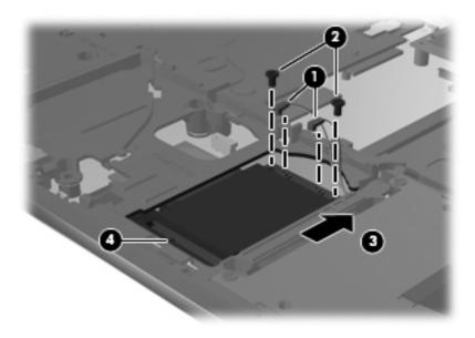
Reverse this procedure to install the WLAN module.
