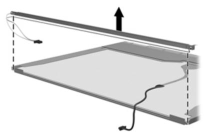
17. Remove the backlight from the backlight frame.
