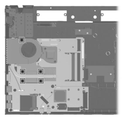
Where used: 5 captive screws that secure the heat sink to the system board
