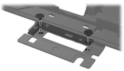
Where used: 2 screws that secure the button board to the switch cover
