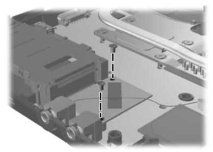
Where used: 2 screws that secure the modem module to the computer
