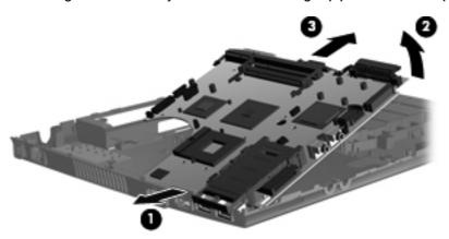
9. Turn the system board upside down with the rear panel toward you to disconnect the power cable.
