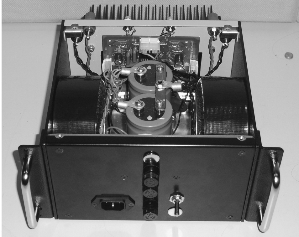
Figure 1. Complete LM4702-Based 100W/Channel High-Fidelity Power Amplifier
